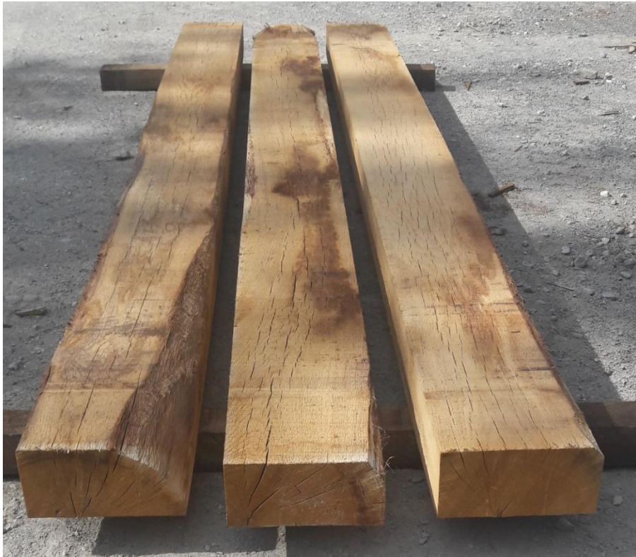
“Rustic” edges on typical sample of sleepers
